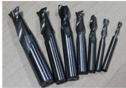
Fluted Hss end mill 4-16mm
